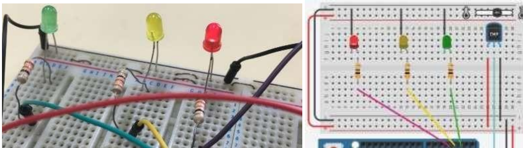
Figure 13- Red LED Function Check (temperature below 15°C or above 35°C)
