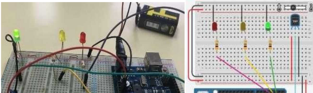
Figure 11 - Green LED Operation Check (temperature between 20 and 30 ° C)
