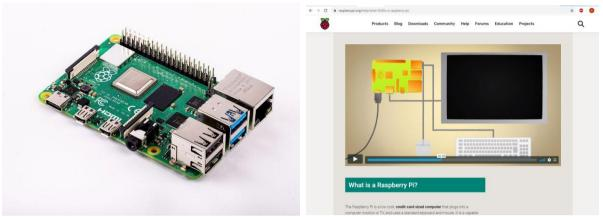
A low-cost Linux and ARM-based computer on a small circuit board sponsored by the charitable Raspberry Pi Foundation in the U.K.
