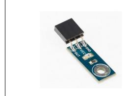
This is a brick component specially designed for the Arduino board, used to measure the environment light level.
