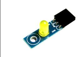
A LED brick is the easiest way to make light using an Arduino. A LED brick needs a spare digital PIN so it can be controlled by the Arduino.
