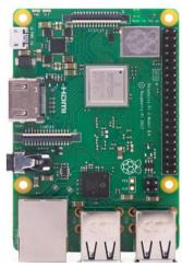
The entire robot is controlled by the Raspberry Pi3 B + development board, which in turn controls other development boards via the I2C (Inter-Integrated Circuit) digital pins.
